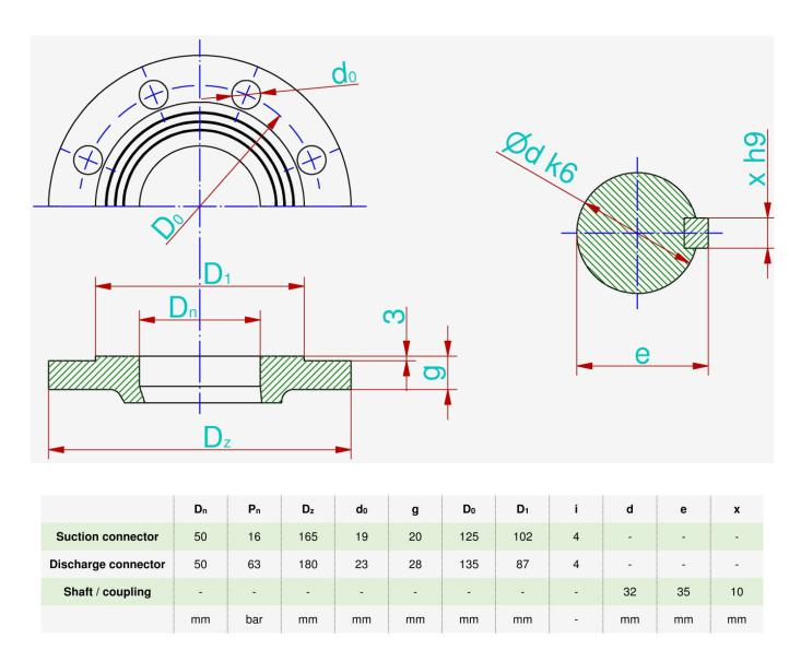
The flanges are normally made in accordance with the standard PN-EN 1092-1 or PN-EN 1092-2.
