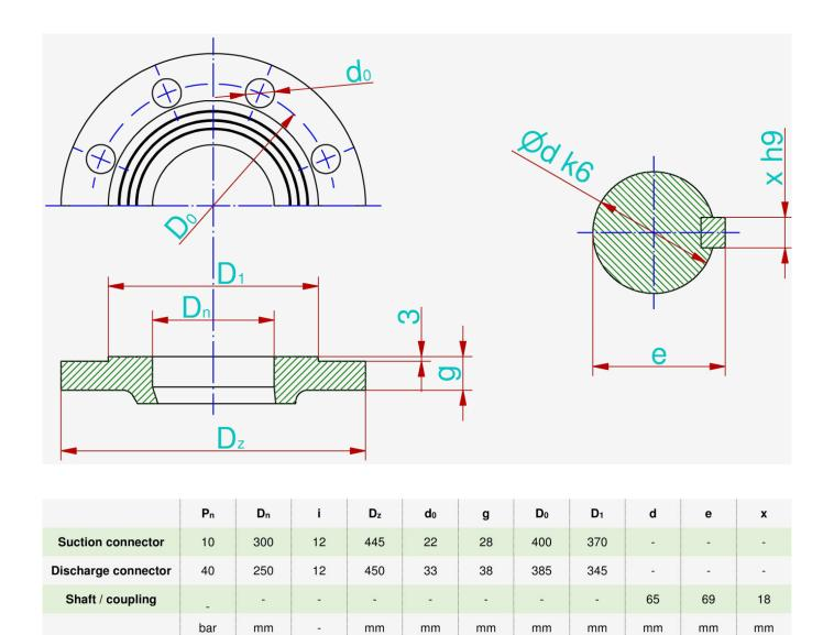
The flanges are normally made in accordance with the standard PN-EN 1092-1 or PN-EN 1092-2.
