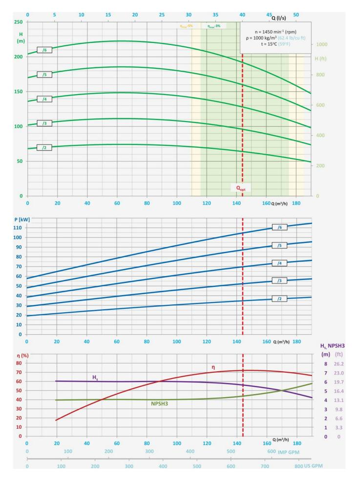
• H = f(Q) – lift head acc. to rate flow,
